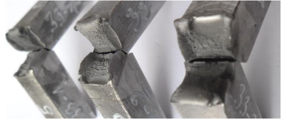
Fig. 14. Appearance of fracture surface after testing of samples notched at fusion zone
