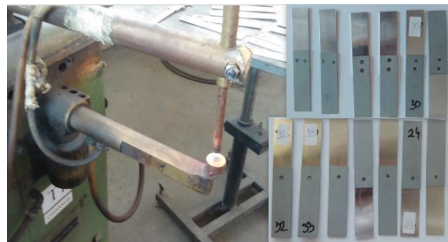
Fig. 4: Spot weld machine and specimen after spot welding
