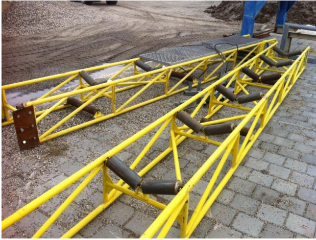
Fig.12: Carrying structure of the belt conveyor at the working site
