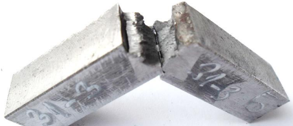
Fig. 8. Sample with V-notch at welded joint after testing of impact toughness
