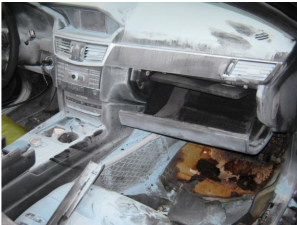
Fig.3: Showing the inside of the vehicle affected by fire
