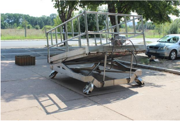
Fig.6: Implemented technical solution of the work platform for maintenance of penstock – position 2
