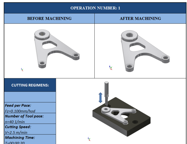
Fig. 11: Operation sheet grooving
