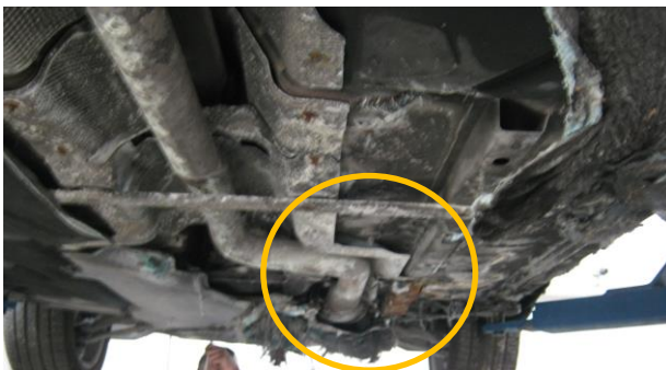
c) front lower part of the vehicle - a place where fire occurred, "fire center"
