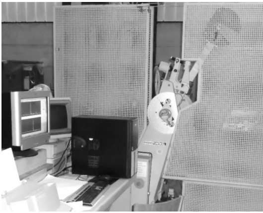
Fig. 5. Computerized Charpy pendulum used for testing
