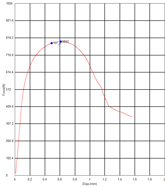
Fig. 7: Force/displacement diagram for the E24 specimen
