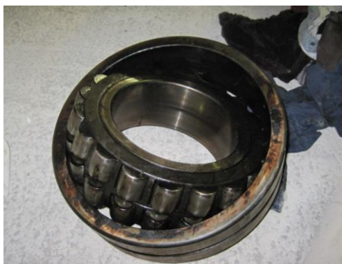
Fig.12: Visible traces of skidding on inner ring
