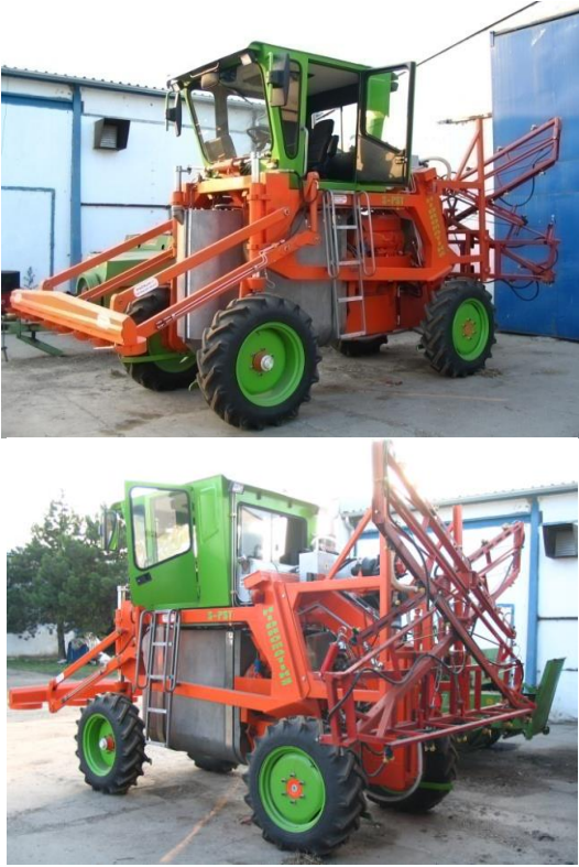
Fig. 1: Self-propelled agricultural machine with high clearance Hidromatiks S-PST
