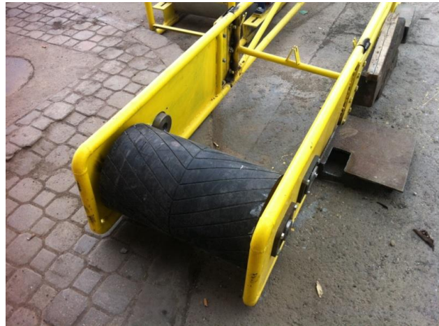
Fig.10: The drive pulley mounted on the belt conveyor carrying structure
