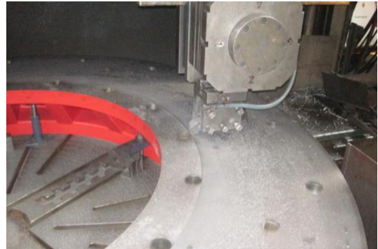
Fig.5: Machining of bearing plate
