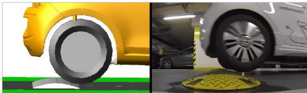
Fig.10: Comparison of simulation and camera record
