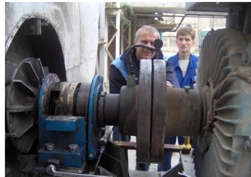
Fig.10: Misalignment measurement on coupling
