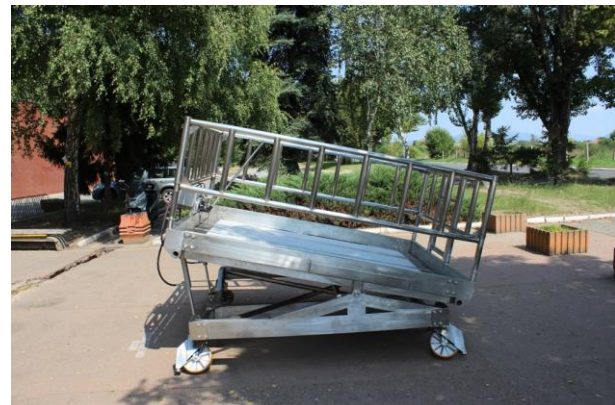
Fig. 5: Implemented technical solution of the work platform for maintenance of penstock – position 1
