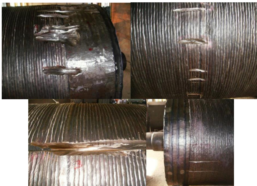
Fig.3: Some of the cracks on the treiber rolls after the surfacing
