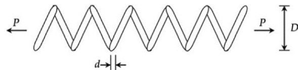
Fig.3: Schematic view of tension/compression spring problem
