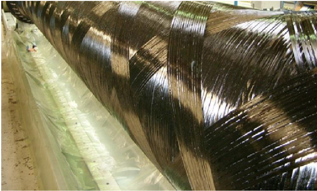
Fig.2: manufacture of composite shaft with FW machine
